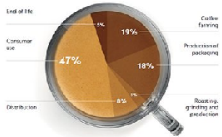
Life Cycle Assessment of a cup of Nespresso Espresso in 8 oz paper cup (Quanta, LCA 2009)
